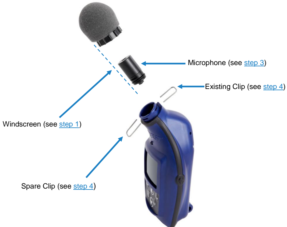
Figure 6-1: Microphone and windscreen assembly
