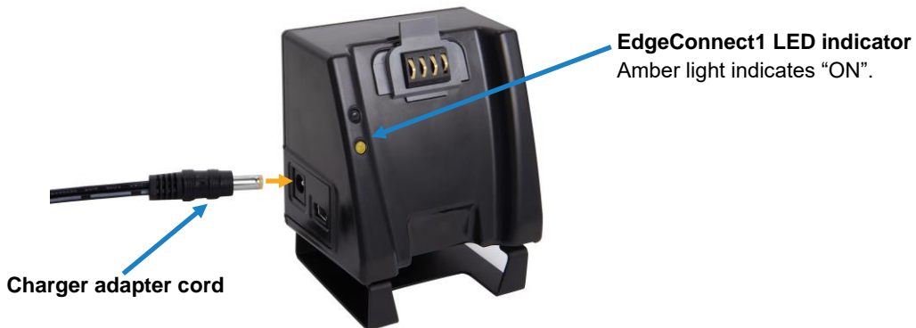
Figure 2-5: Attaching charger adapter to EdgeConnect1 (use EdgeDock1 for models EG3, EG4, EG5)
