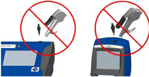
Figure 4-3: Do NOT Blow into Instrument
